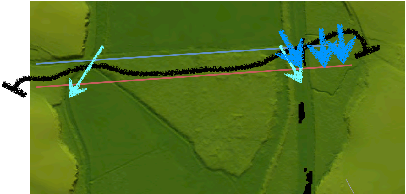
Figure 27: Annotated sketch of road route through refuse site and key drainage culverts for drainage of the northern section of big marsh. Option C
